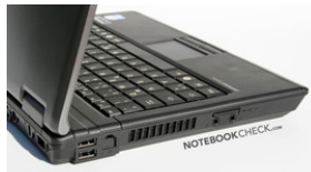
Left side: Headphones, microphone, cardreader, modem (not built in here), 2x USB
